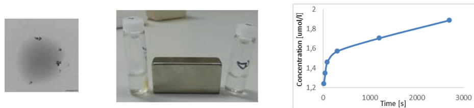
Figure 1 – Magnetoliposome (left), aggregation of magnetoliposomes near permanent magnet (middle), releasing of DOX caused by alternating magnetic field (right)
